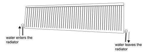
The radiator is full of water which flows from a boiler through the radiator and back to the boiler.
