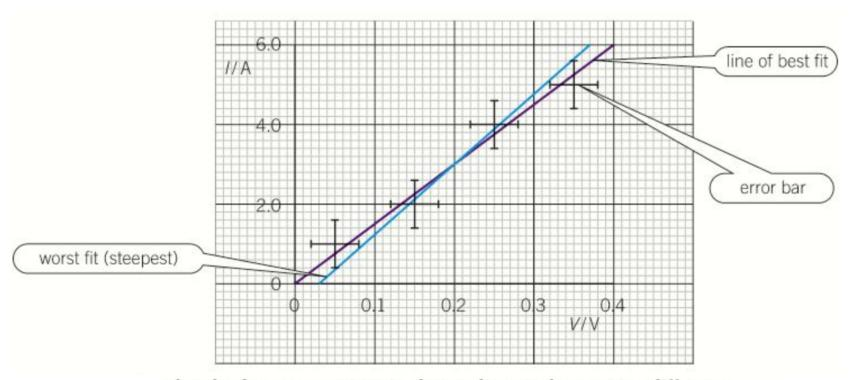
The absolute uncertainty in the gradient is the positive difference between the gradient of the line of best fit and the gradient of the line of worst fit.
