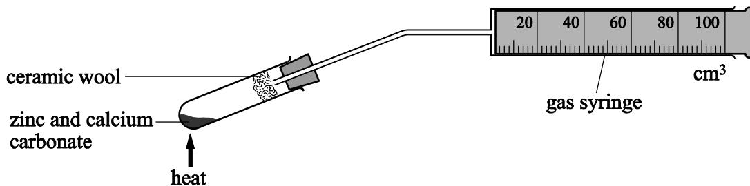
A mixture containing 0.27 g of powdered zinc and 0.38 g of powdered  $\text{CaCO}_3$  was heated strongly for two minutes. The volume of gas collected in the  $100 \text{ cm}^3$  syringe was then measured. The experiment was then repeated.
